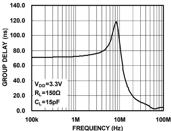
Figure5. Group Delay vs Frequency (SD Channel)
