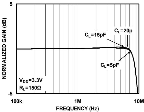
Figure3. Gain Vs. Frequency With CLOAD (SD Channel)
