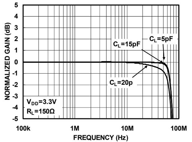
Figure4. Gain Vs. Frequency With CLOAD (FHD Channel)
